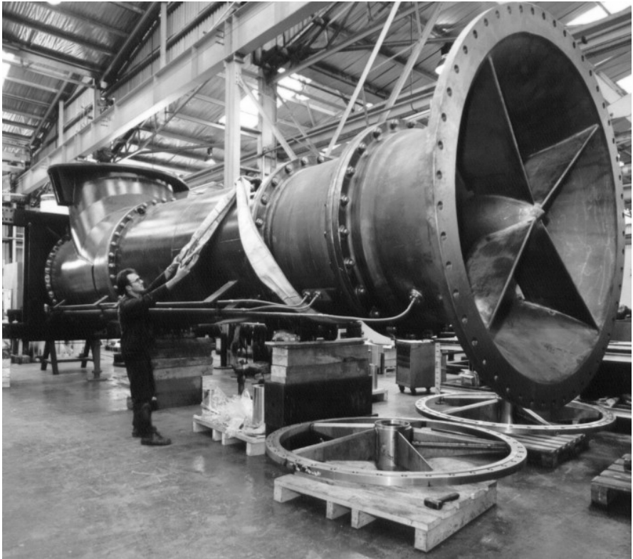
Semi-axial cooling water pump, Sulzer Pumps
