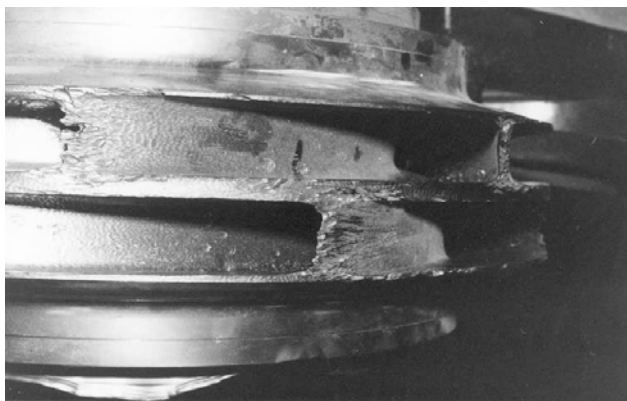
Fig. 14.27. Hydro-abrasive wear at the outlet of a double-entry impeller
