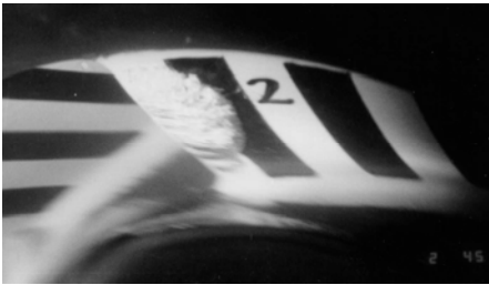
Fig. 6.11. Cavity at the impeller blade leading edge
